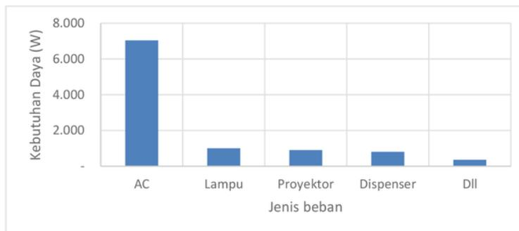
**Figure 1.** Energy demand of Refrigeration Laboratory Building
