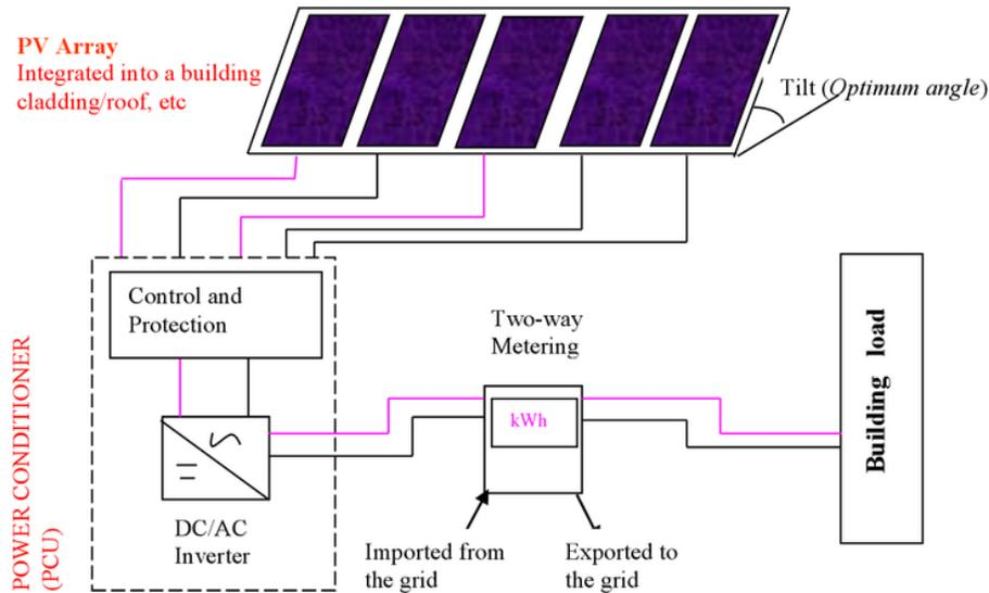
**Figure 2.** Building Integrated Photovoltaic design
