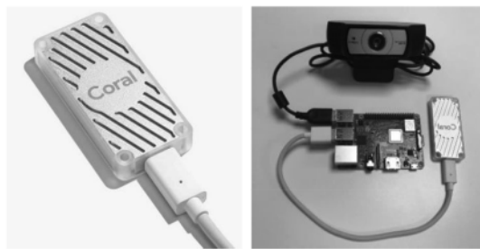
(a) Coral USB Accelerator (b) Raspberry Pi, Webcam and Coral Fig. 11. Embedded devices for object detection.
